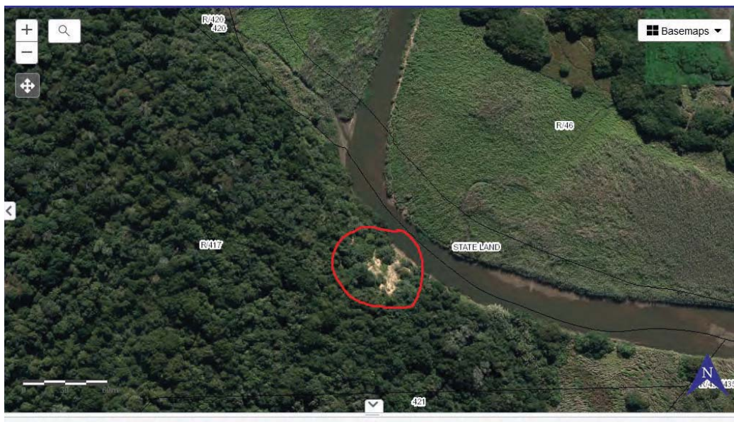
Fig. 1c. An aerial perspective of the area taken in 2018/2019 shows a previous slip which would have likely occurred due to a similar rainfall or disturbance event. The erosion site is located on the outer-apex of the river bend so this may be part of ongoing catchment-scale processes.
